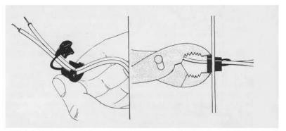
25( ) Separate the two conductors of the line cord from the stripped end to the strain relief, and cut off 9 1/2" (24 cm) from *one* (either) conductor. Strip about 3/8" (1 cm) of insulation from the short-cut conductor, and connect it to power fuse holder lug #2 (S). Position the other (long) conductor against the chassis on the left side. This conductor will be connected later.
