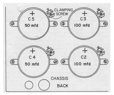
torial Diagram. Now install the two 100 mfd capacitors in the other brackets. Position the (+) terminals toward the front, and tighten all clamps and mounting hardware.
